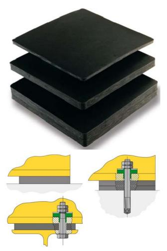
\*Where bolt through connections are required, Farrat Anti-vibration (AW) washers and bushes should be incorporated in order to allow free movement of the pad and to ensure that the bolt does not transmit vibration across the connection.
